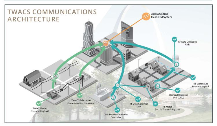
The TWACS power line communication system offers bi-directional and concurrent transmission of data, capturing more that 99% of device readings.
